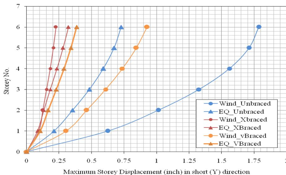
**Figure 4:** Lateral storey displacement in short direction
