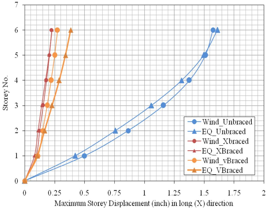
**Figure 5:** Lateral storey displacement in long direction
