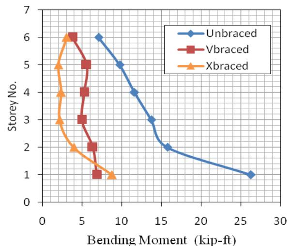
**Figure 9:** Bending moments in 1A-corner column **Figure 10:** Bending moments in 2A-exterior column
