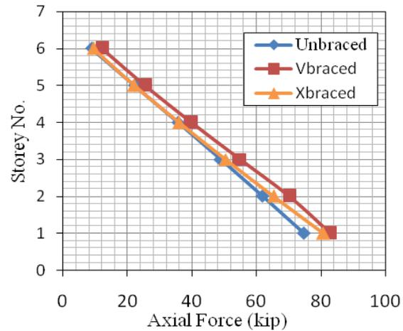
**Figure 7:** Axial forces in 1A-corner column **Figure 8:** Axial forces in 2A-exterior column
