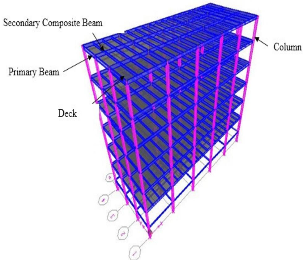
**Figure 2:** 3D view of steel building without bracing
