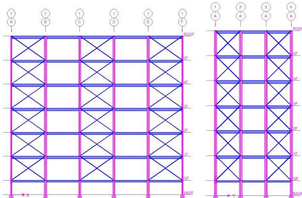
**Figure 3a:** Concentric bracing in long direction
