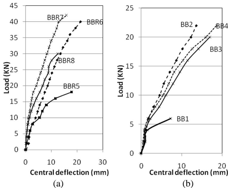
**Figure 5:** Comparison of different web reinforcement
