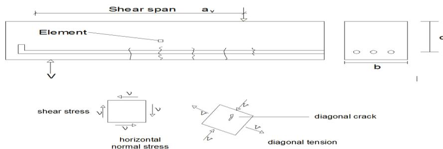
**Figure 2: Stresses on an element in concrete beam**
