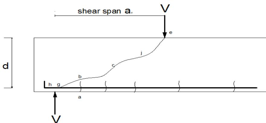
**Figure 6:** Crack development in beams
