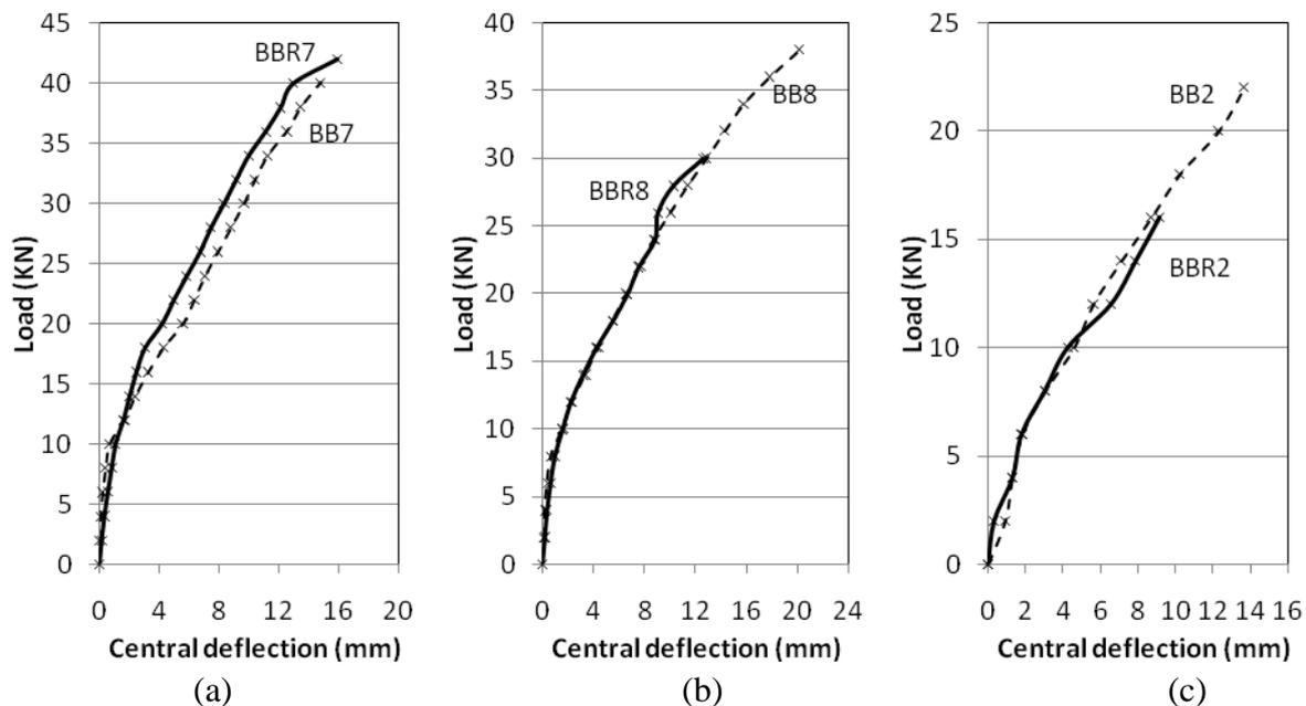
**Figure 4:** Typical load deflection curves of tested beam
