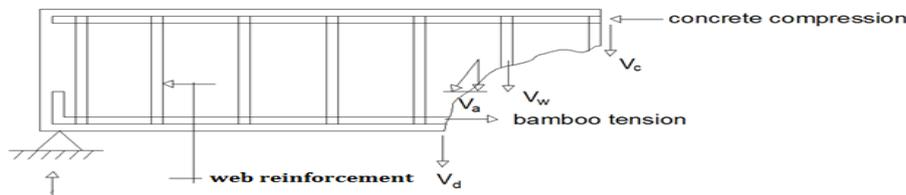
**Figure 1: Shear transfer in beam with web reinforcement**
