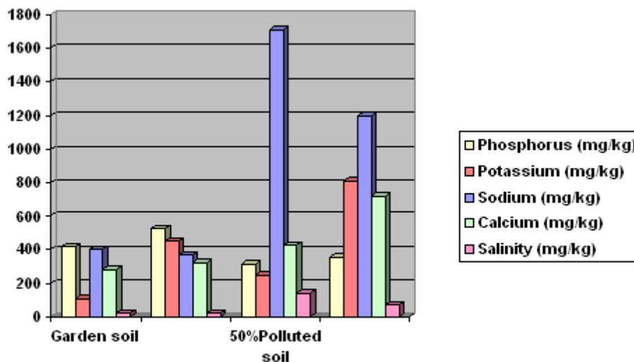
**Figure 1:** A few physico-chemical characteristics of the various soil samples
