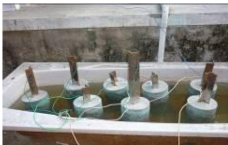
Fig: 7 Externally Coated by FACSR Specimens Coated Specimens
