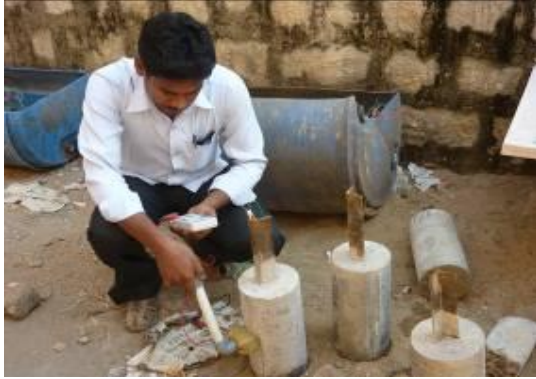
Fig:5: Half Cell test in Specimens
