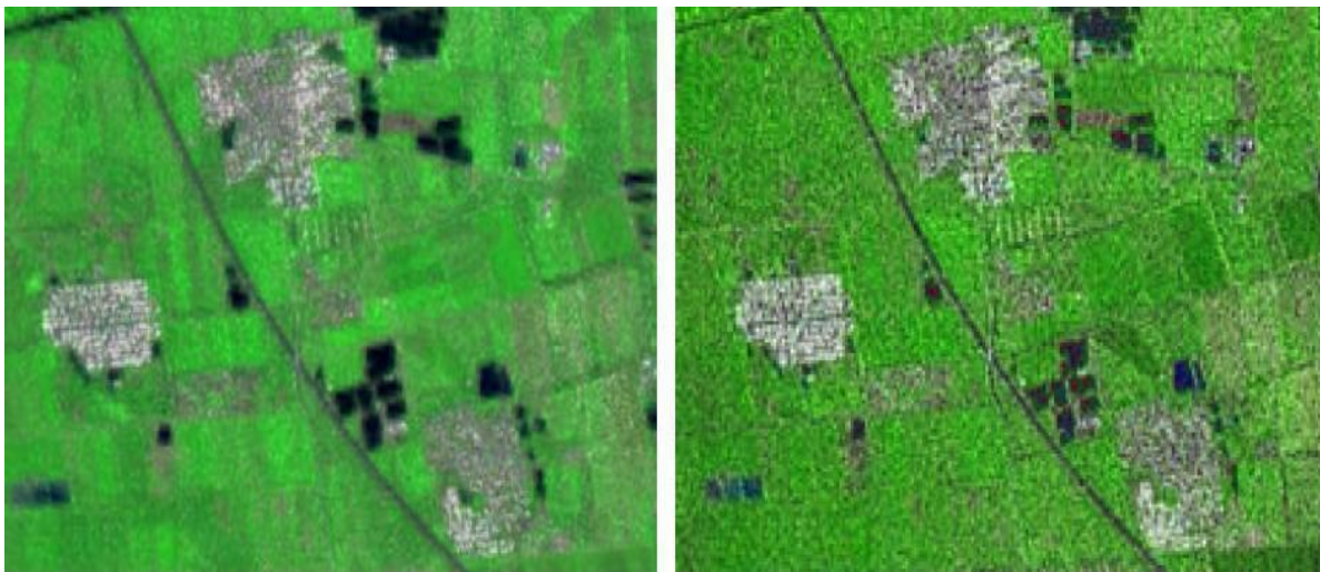
Figure 4: Examples of HIS fused and SAR images (on the left) and Brovey fused TM and SAR images (on the right)
